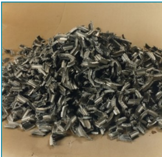
ILW Magnox fuel cladding swarf
