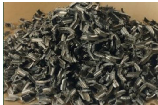
ILW Magnox fuel cladding swarf
