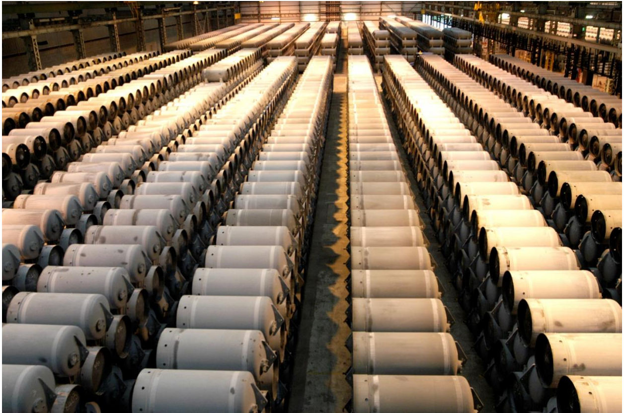
Uranium hexafluoride cylinders at Capenhurst
